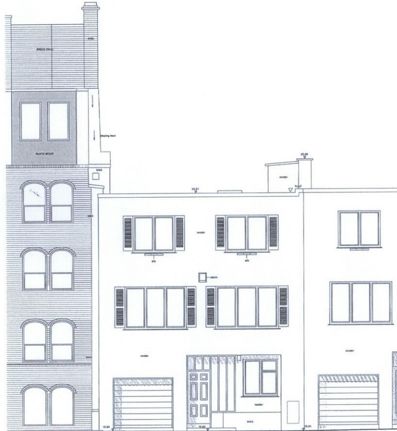
Existing Front Elevation
